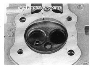
Check the cylinder head for warpage with a straight edge and feeler gauge.
