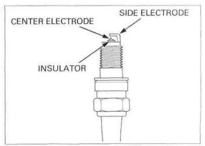
Replace the plug if the center electrode is rounded as shown.
