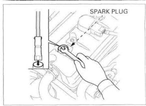
The spark plugs are equipped with iridium type center electrodes. Do not clean the electrodes.
