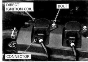
Clean around the spark plug bases with compressed air before removing the plugs, and be sure that no debris is allowed to enter the combustion chamber.
