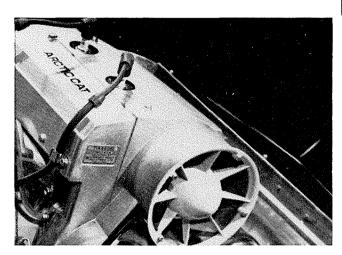
The above described numbers are required to properly complete warranty claims and to insure the correct replacement parts are obtained. Under no circumstances should warranty be allowed if the chassis model and serial number plate has been tampered with or removed. If a new engine is installed, notify the distributor and the factory of the new engine model and serial number.
