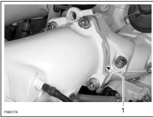
1. Torque Allen screws and nut to 40 N•m (30 lbf•ft)
